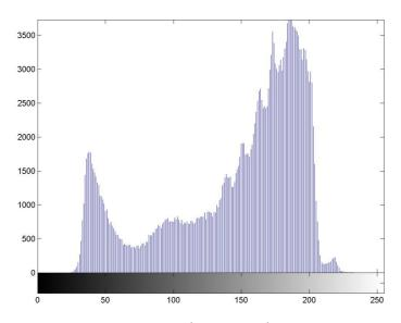
The threshold can be chosen according to different ways. In the case of ISABE\_LUMI image, the histogram presents two peaks around the gray levels 75 and 190. We can then for example choose the median gray level between these two peaks as threshold. Nevertheless there are many other ways to choose the threshold: intensity mean value of the histogram, median value of the full gray level range [ 0, 255 ])...
