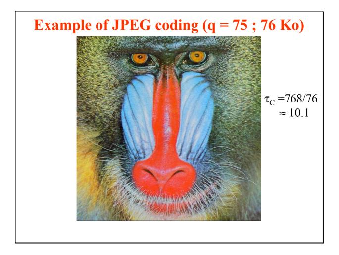
Finally, the image above presents a result where the image quality is paramount over the compression. The number of bits required to store the encoded image is 10 less than what is required to store the original image. It is however difficult for the human eye to detect the loss of picture quality: it is hard to differentiate between this and the original image in terms of the color range and the sharpness of colors and textures.
