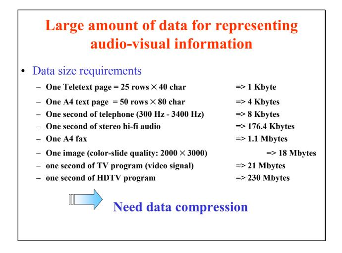
To illustrate the problem that a large quantity of data are required to represent a little information from an image signal, the document above gives an indication of the data sizes required to store and transmit different images, that we regularly find in our environment. These use Anglo-Saxon units, so remember that 1 byte = 1 octet = 8 bits.
