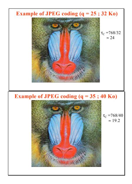
Two more results obtained by giving precedence to image quality rather than the compression rate. However, this time, the compression rate was divided by only 1.25. The evolution of the compression rate according to the quantization is generally not a linear function.
