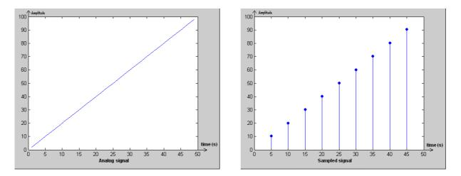
The figure above represents a ramp type signal before and after sampling. The sampling frequency equals 0.2Hz  $(\frac{1}{5}s^{-1})$ . The amplitude of this signal varies continuously over the interval [0, 100], so a quantification will be necessary.
