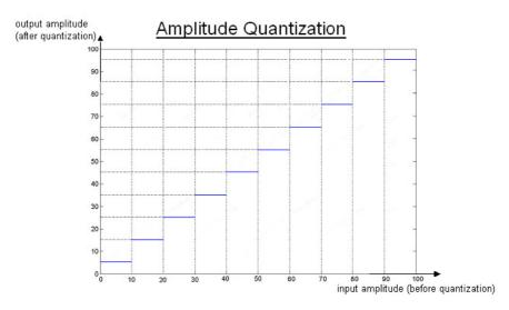
The figure above represents an example of quantification: if a sample of the signal has an amplitude included in the interval [10k; 10(k+1)], « k » being a natural integer, the amplitude value would be brought by quantification to 10k+5.
