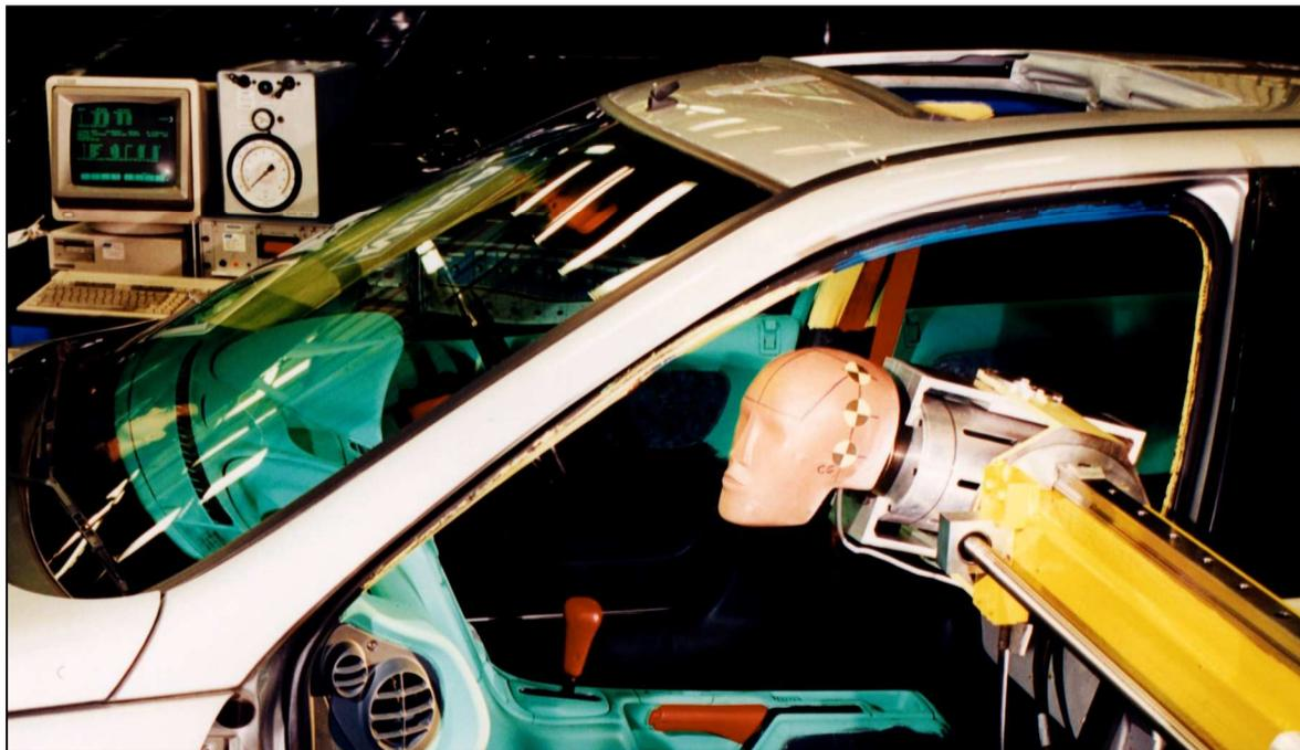
MIRA's Headform Impact Test System (HITS) for FMVSS 201 validation.
