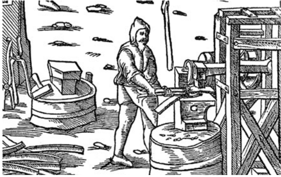
Fig. 1.1 Medieval powered hammer for metal working. From: Georgius Agricola, De Re Metallica , Basel 1556
